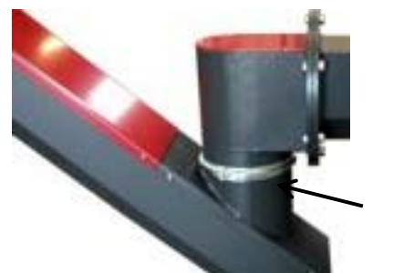
Auger fixed to outlet of scraper system by means of the pipe-clamp
