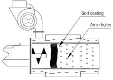
Fig. 4 - Maintenance of burner tube
