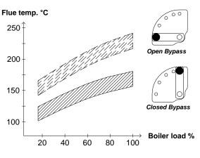
Fig. 3- Approx. flue temperature compared to boiler load
