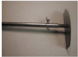
Scraper (only by boilers with stoker in rear)
